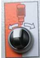
Fig. 13: Selection switch in middle position
