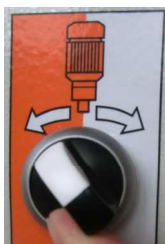
Fig. 14: Selection switch in left position
