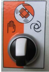
Fig. 10: Selection switch setting "0"
