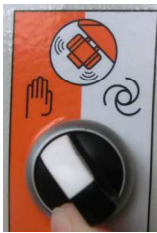
Fig. 11: Selection switch setting "Manual"
