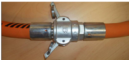
Fig. 40: Detaching connections
