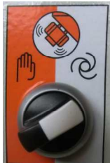
Fig. 12: Selection switch setting "Automatic"
