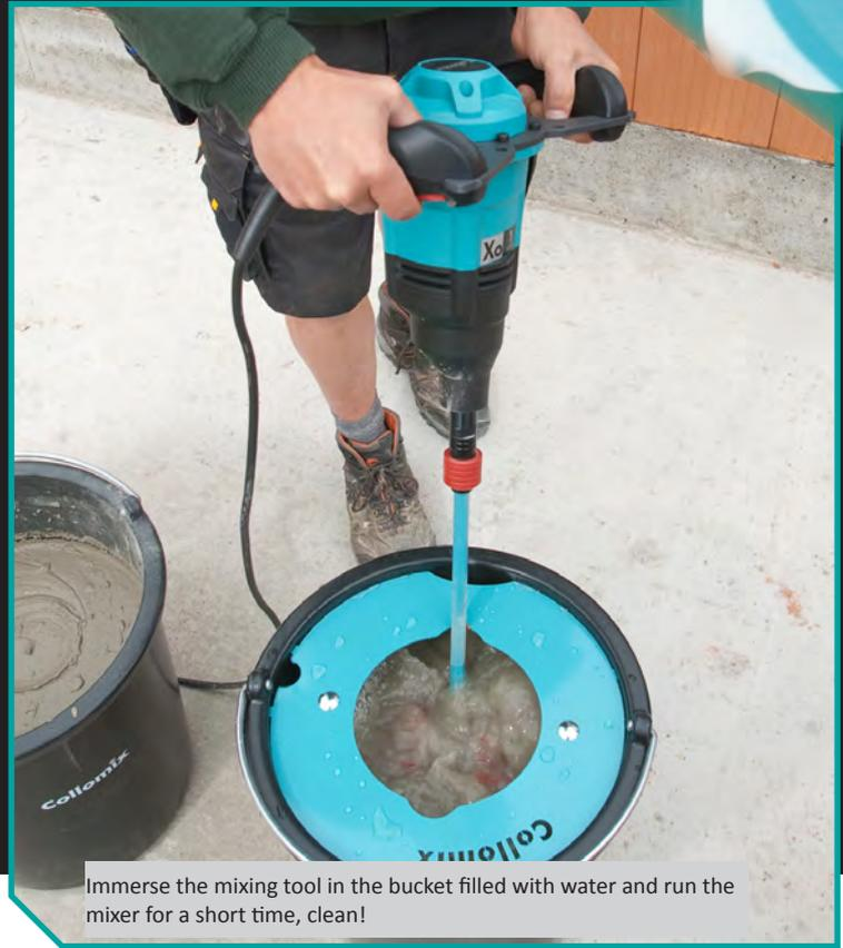
Immerse the mixing tool in the bucket filled with water and run the mixer for a short time, clean!
