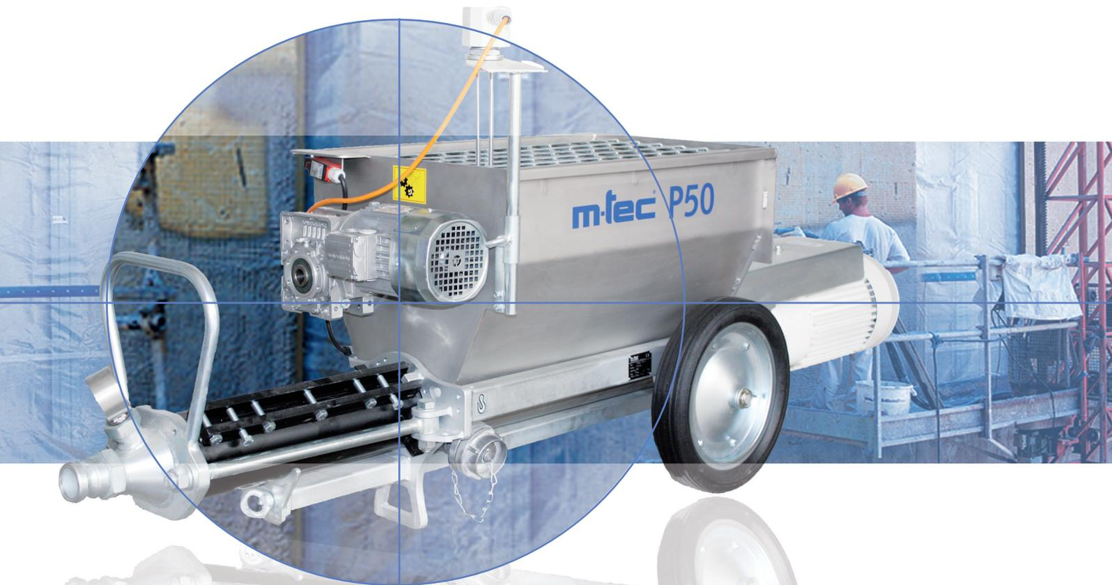
The m-tec P50 is a powerful mortar pump for conveying all pumpable product with a max grain size up to 8 mm. Therefore the P50 is the perfect machine for processing mortars, concretes, plasters as well as self leveling compounds and floor screeds. The P50 is available in different designs suitable for the different applications with an output up to 110 l/min.
